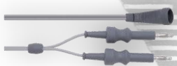
SILICONE BIPOLAR CABLE 10' (3.0 M) 190-100 Instrument Connector: USA 2-Pin Plug Generator Connector: 4mm Banana Plug Compatibility: Valisels, Conwell, Colson, Olympus & Most Bipolar Generator
